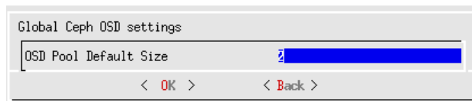
Figure 9.9: Ceph Installation OSD Global Settings: OSD Pool Default Size
