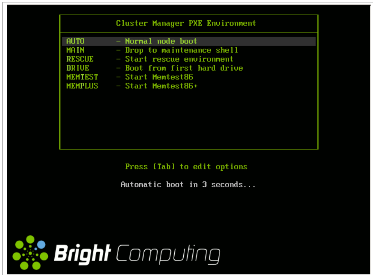
Figure 5.15: PXE Menu With Install-mode Set To AUTO
