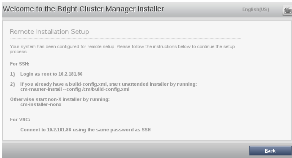
Figure 3.5: Remote Installation: VNC and SSH access explanation
