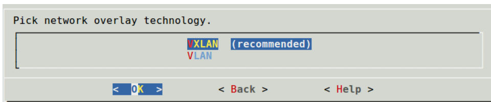
Figure 1.9: Setting VXLAN as the network overlay technology
