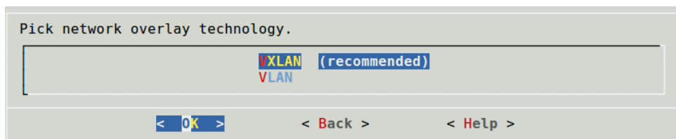
Figure 1.10: Setting VXLAN as the network overlay technology
