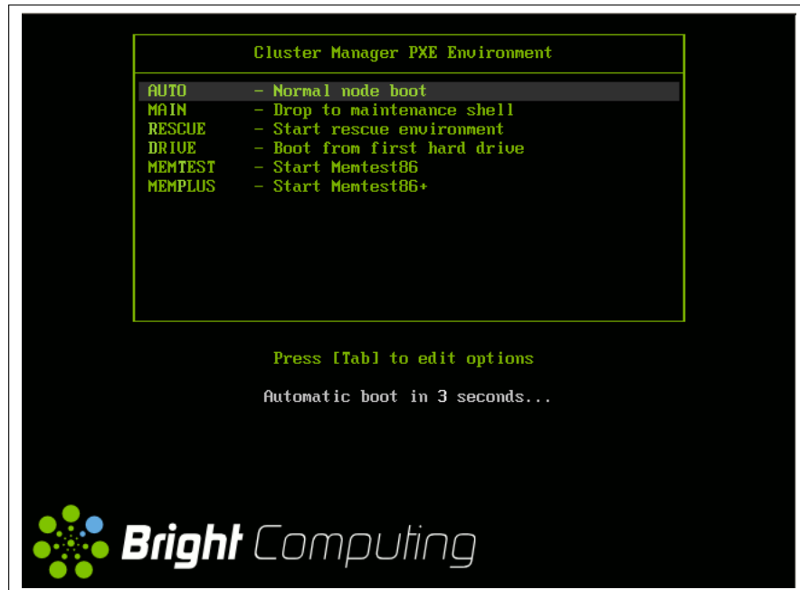
Figure 6.17: PXE Menu With Install-mode Set To AUTO
