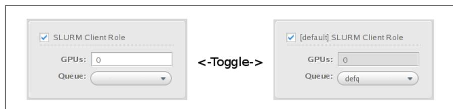
Figure 8.5: Workload Management Role Assignment Toggle States For An Individual Node
