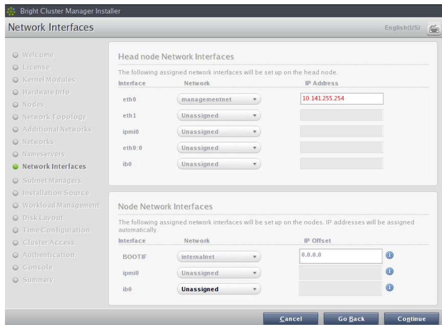
Figure 2.14: Network Interface Configuration: *type 3*
