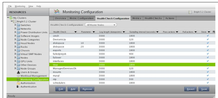
Figure 10.27: cmgui Monitoring: Health Check Configuration Display After Category Selection
