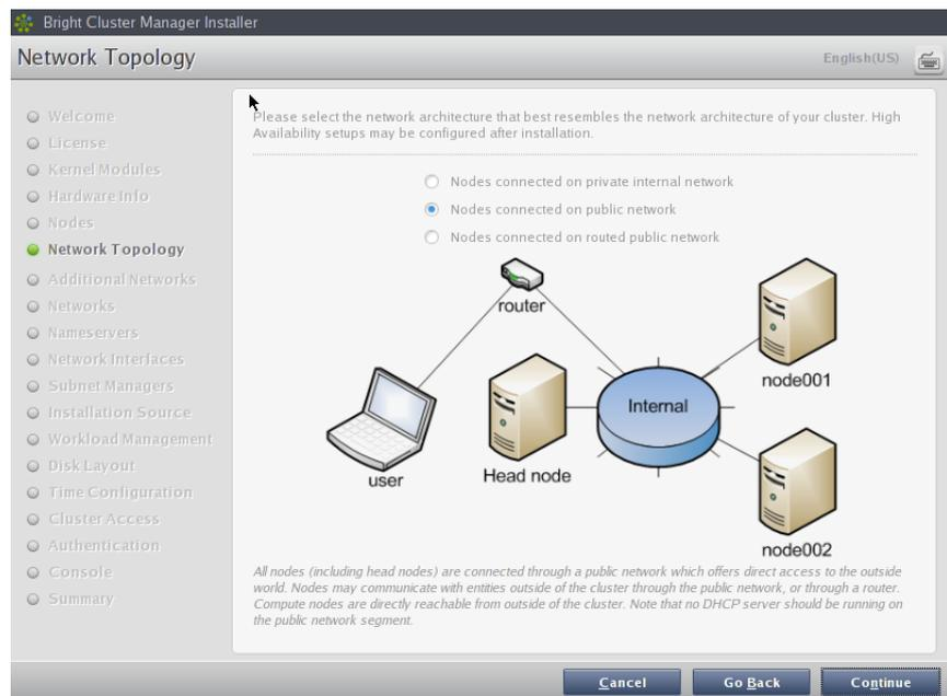
Figure 2.8: Networks Topology: nodes connected on a public network
