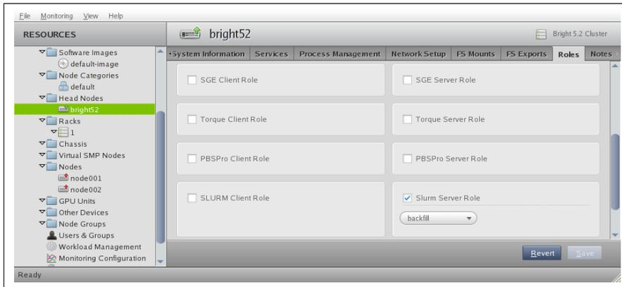
Figure 8.2: Workload Management Role Assignment On A Head Node
