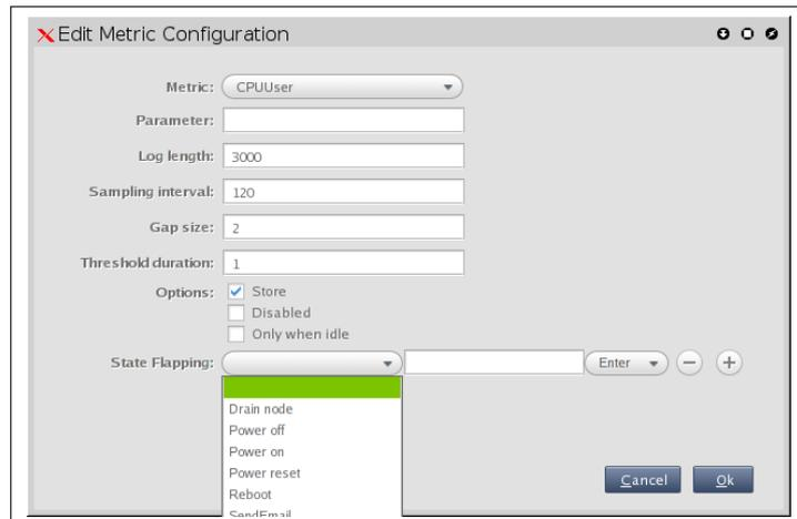
Figure 10.22: cmgui Monitoring: Metric Configuration Tab Edit Dialog
