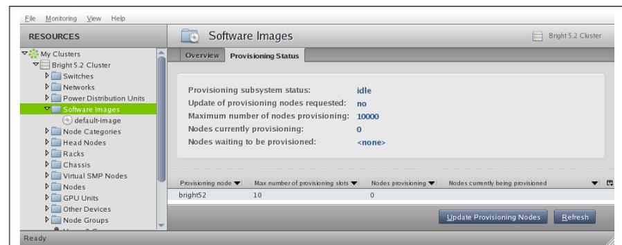
Figure 6.3: `cmgui`: A Button To Update Provisioning Nodes
