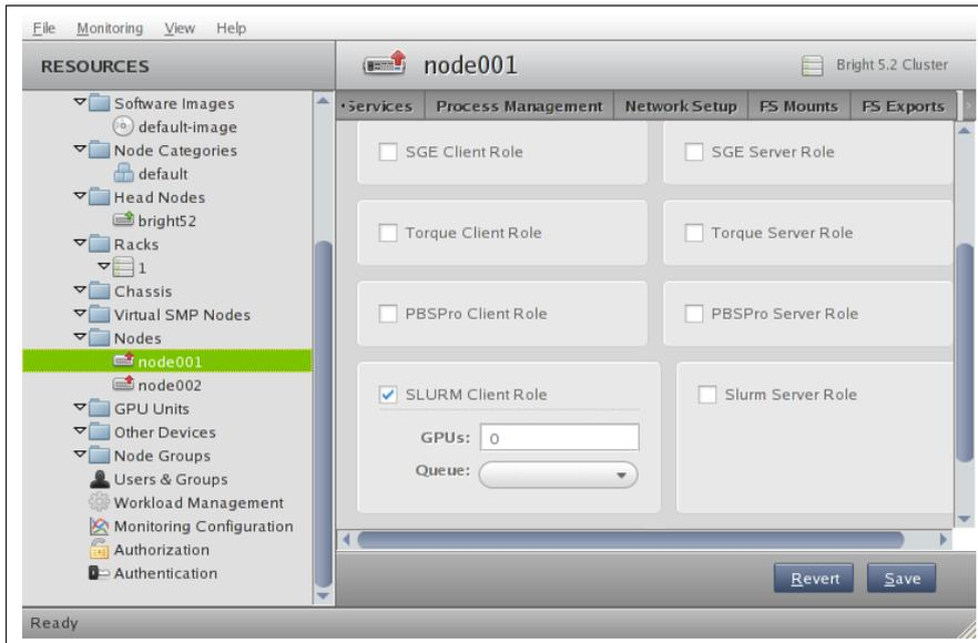
Figure 8.4: Workload Management Role Assignment For An Individual Node
