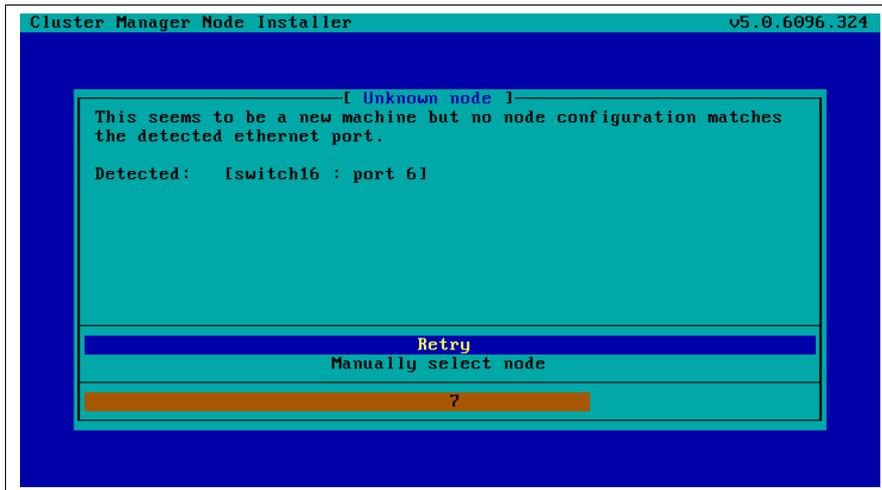
Figure 6.8: Scenarios: Unknown Node, Ethernet Port Detected
