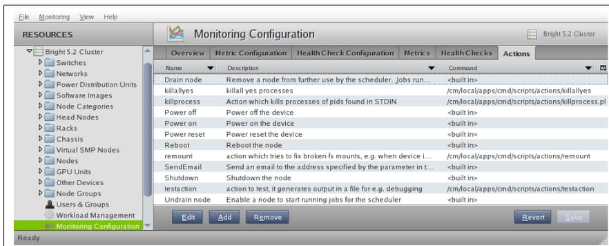
Figure 10.33: cmgui Monitoring: Actions Tab
