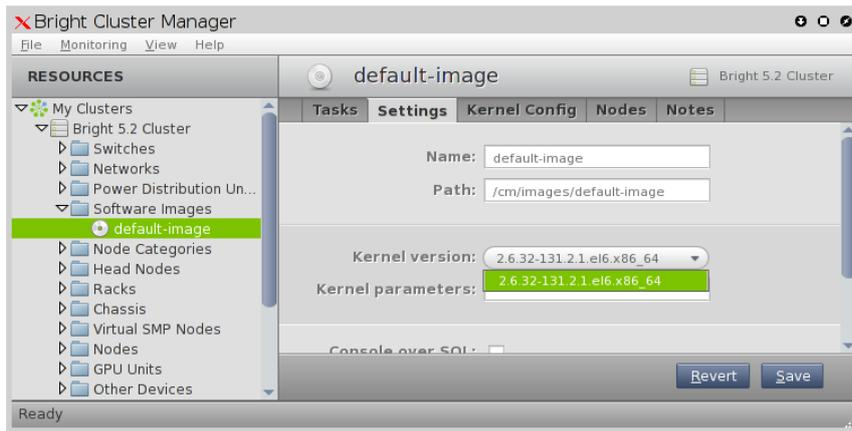
Figure 9.1: Updating A Software Image Kernel In cmgui
