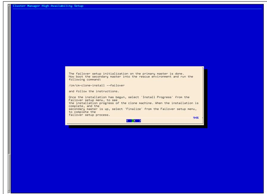
Figure 13.4: cmha-setup Instructions To Run On Secondary For Cloning
