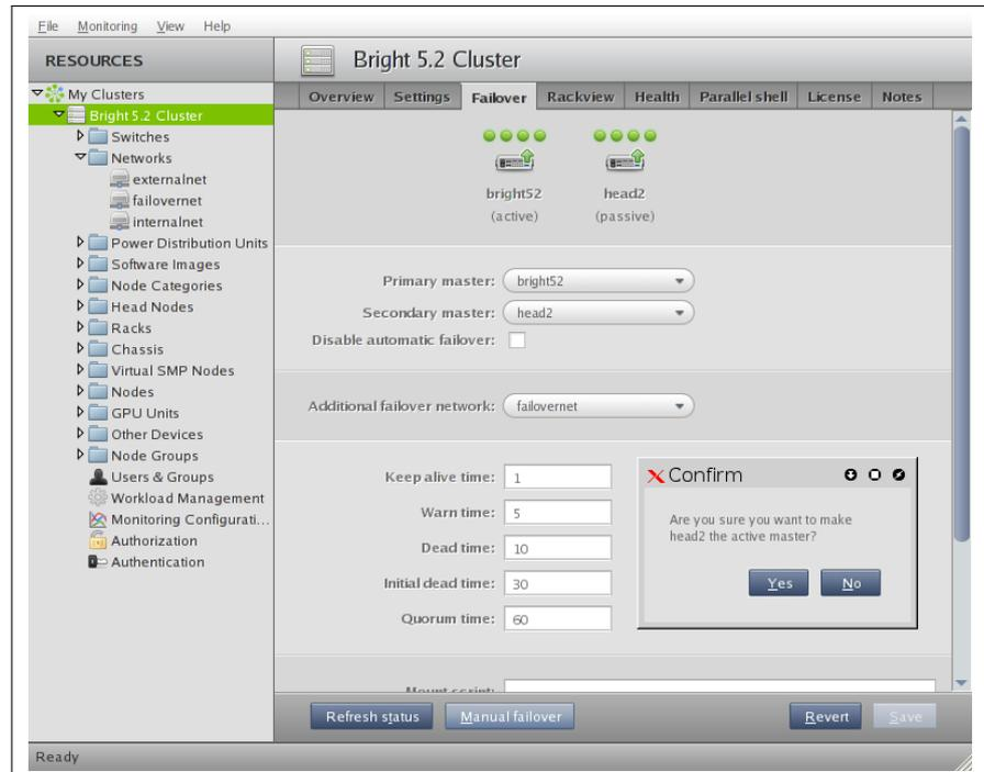
Figure 13.7: Accessing HA Cluster Parameters And Functions Via cmgui
