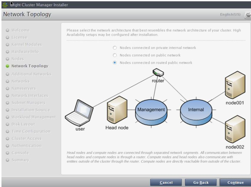
Figure 2.9: Network Topology: nodes connected on a routed public network
