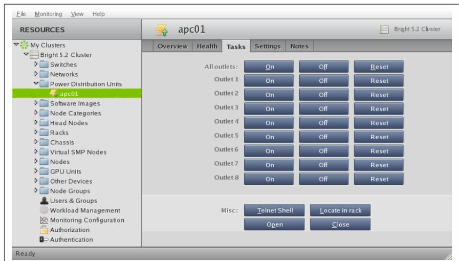
Figure 5.5: PDU Tasks
