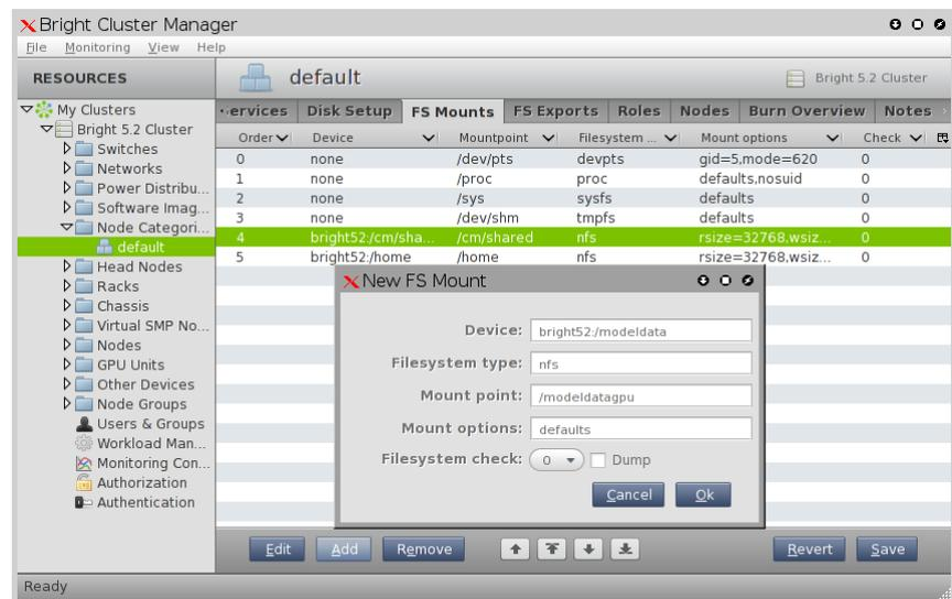
Figure 4.14: Setting Up NFS Mounts On A Node Category Using `cmgui`
