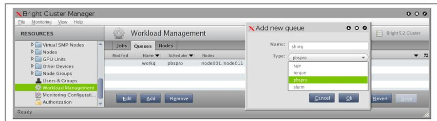
Figure 8.13: Adding A New Queue Via cmgui
