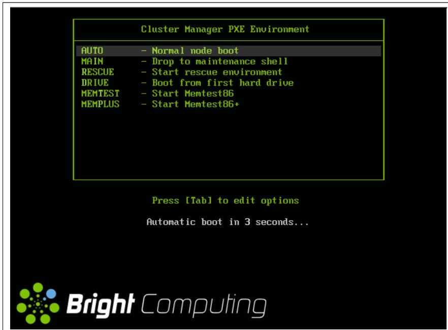
Figure 6.15: PXE Menu With Install-mode Set To AUTO
