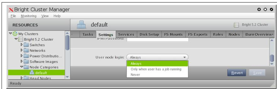
Figure 8.1: Disallowing User Logins To Nodes Via `cmgui`
