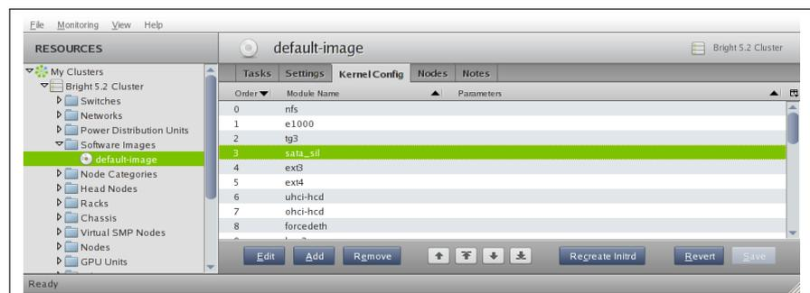
Figure 6.4: `cmgui`: Selecting Kernel Modules For Software Images
