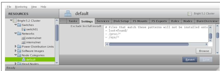
Figure 6.19: Setting up exclude lists with `cmgui` for provisioning
