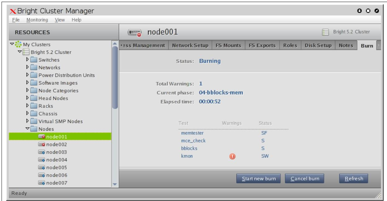
Figure N.2: cmgui: Status Of A Burn Run—Node View
