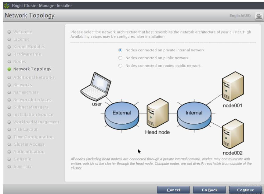
Figure 2.7: Networks Topology: nodes connected on a private internal network
