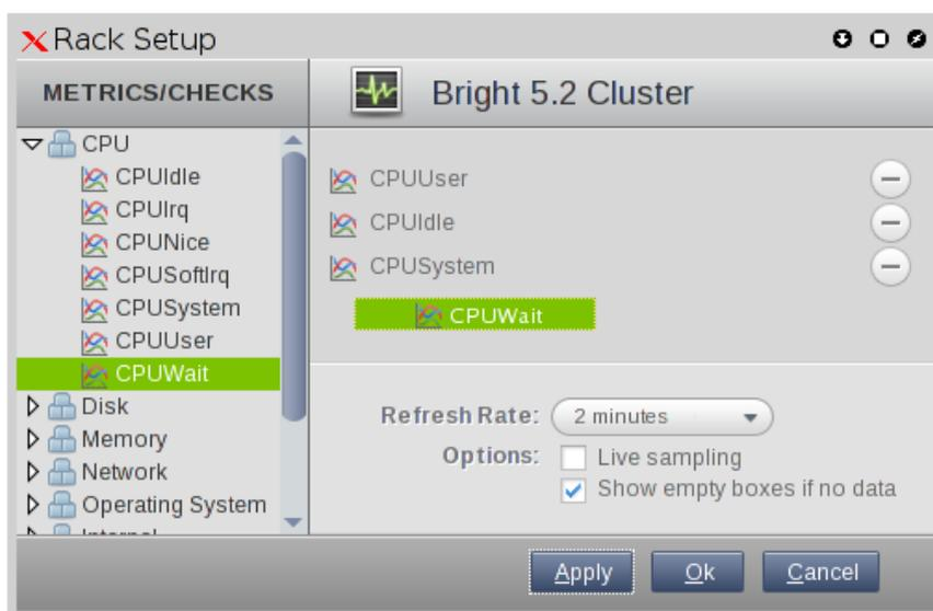
Figure 4.22: Rack Setup, Showing Drag-And-Drop Of CPUwait Metric
