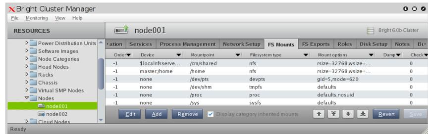
Figure 4.15: Display Of Category Inherited Mounts In cmgui
