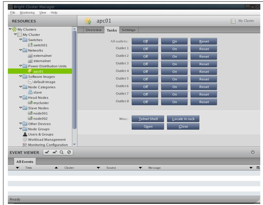
Figure 5.5: PDU Tasks
