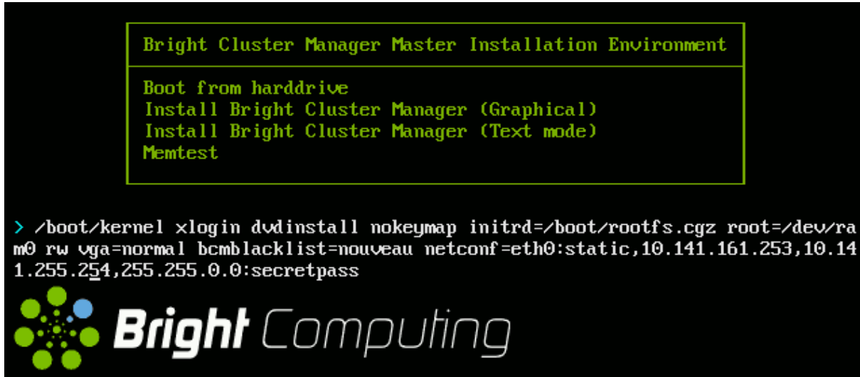
Figure 3.1: Installation: ISO Boot Menu For Legacy BIOS
